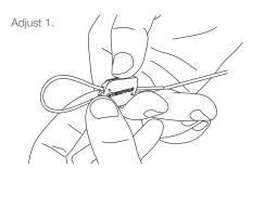
Ensure a minimum 75 mm of tail wire exit the hanger.
