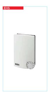
Electronic temperature controller for electric heater batteries up to 3.5 kW (230 V)/6.4 kW (400 V) Type EHS Ref. no, 5002
