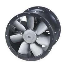
Range of cylindrical cased axial fans fitted with aluminium impellers and manufactured from high grade rolled galvanised steel and protected against corrosion by cataforesis primer and black polyester paint finish.
