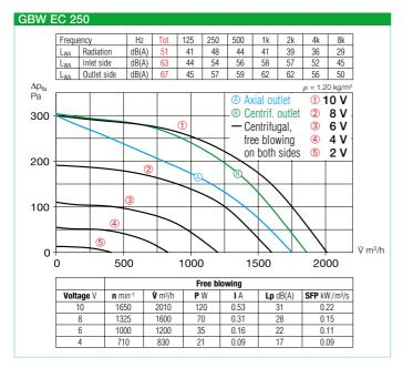
Continuously variable speed control with potentiometer or continuously variable speed regulation with universal control system (see table).
