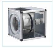
■ With regard to the GigaBox T120 series, the motor is located outside of the air flow and it is separated from the impeller by a thermally insulated wall. The motor-impeller unit can be removed without dismantling the duct system.
